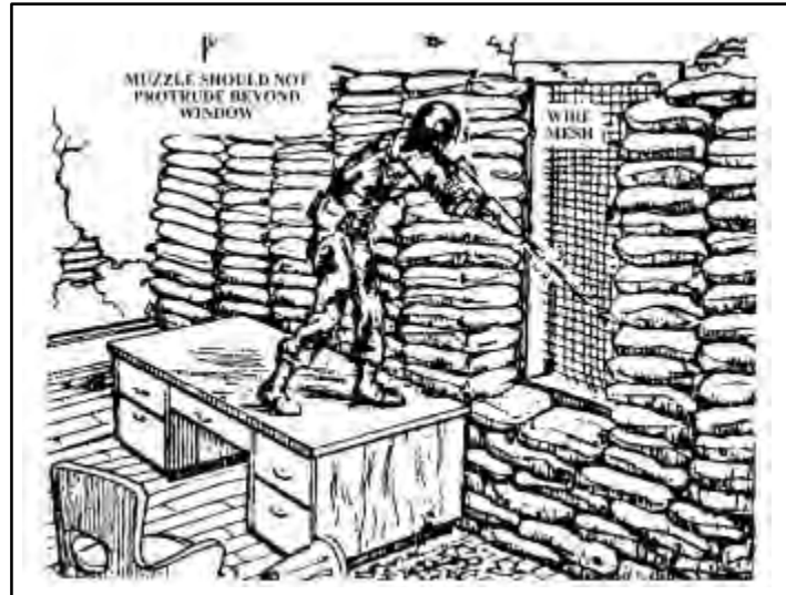
Figure A-56. Window Firing Position
